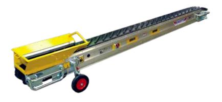
The Shifta is a portable conveyor used for moving rubble, aggregate, soils, concrete, and chippings. It is an aluminium constructed machine, available in 3 lengths and can be easily maneuvered by one person.
