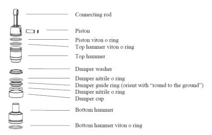
Figure 8: View of the orientation of internal parts.
