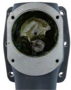
Figure 2: Grease ring example
