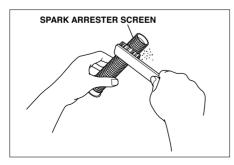
Install the spark arrester, and muffler protector in the reverse order of disassembly.
