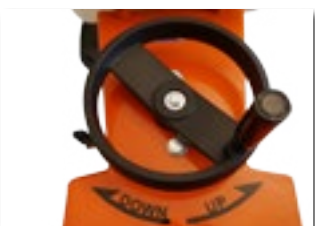
Cutting depth adjustment by handwheel
